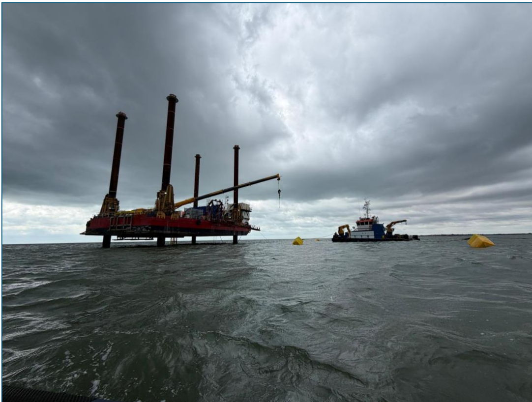
Above image shows the Haven Seachallenger JUB together with a Dive Support Vessel attached to the mooring buoys
